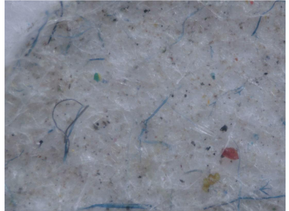
Dust on filter at 220x magnification
